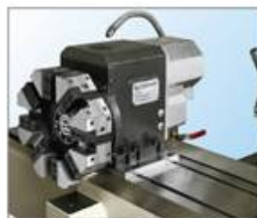
▲ Electrical system Turret
