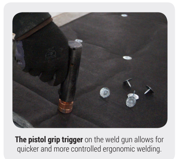
Magnetic tip holds weld pin in place for precision application.
