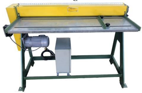
Cut multiple blanks of light gauge sheet metal... in one pass! Great for roofing and architectural! Gang slit blanks from 16 to 30 gauge. Slit blanks at speeds up to 60 FPM Gang slit pre-painted and other sheet material
