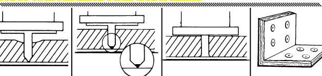
The welding cycle is activated by pressing the trigger switch on the gun. Current flowing through the fastener's high resistance point of contact creates instantaneous welds of extremely high strength.
