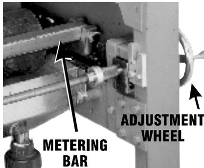
A metering bar accurately controls adhesive application.
