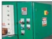
Standard features for the LM1010 control box include: selection for continuous or single cutting stroke, and jog button with reverse switch. A "GO TO" back gauge control pad with stroke counter allows quick, accurate back gauge positioning up to 30 inches.
