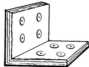
No burn marks or discolorations of duct occur when using the recommended method of insulation fastener attachment. Fasteners are permanently welded in position flush with insulation.
