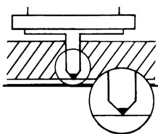
The welding cycle is activated by pressing the trigger switch on the gun. Current flowing through the fastener's high resistance point of contact creates instantaneous welds of extremely high strength.
