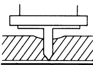
The needle sharp point enables the operator to easily push the fastener through the insulation into firm electrical contact with the metal duct.
