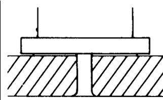
The flow of metal during the weld, firmly attaches and supports the fastener. It prevents breakaway while handling ducts during transport and installation.
