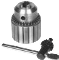
**No. 1897 Key-Type Chuck.** Takes  $\frac{3}{16}$ " (4.76mm) to  $\frac{3}{4}$ " (19mm) drills. Adapts to 3 MT spindle with No. 1898 arbor. 4 lbs. (1.8 kg)
