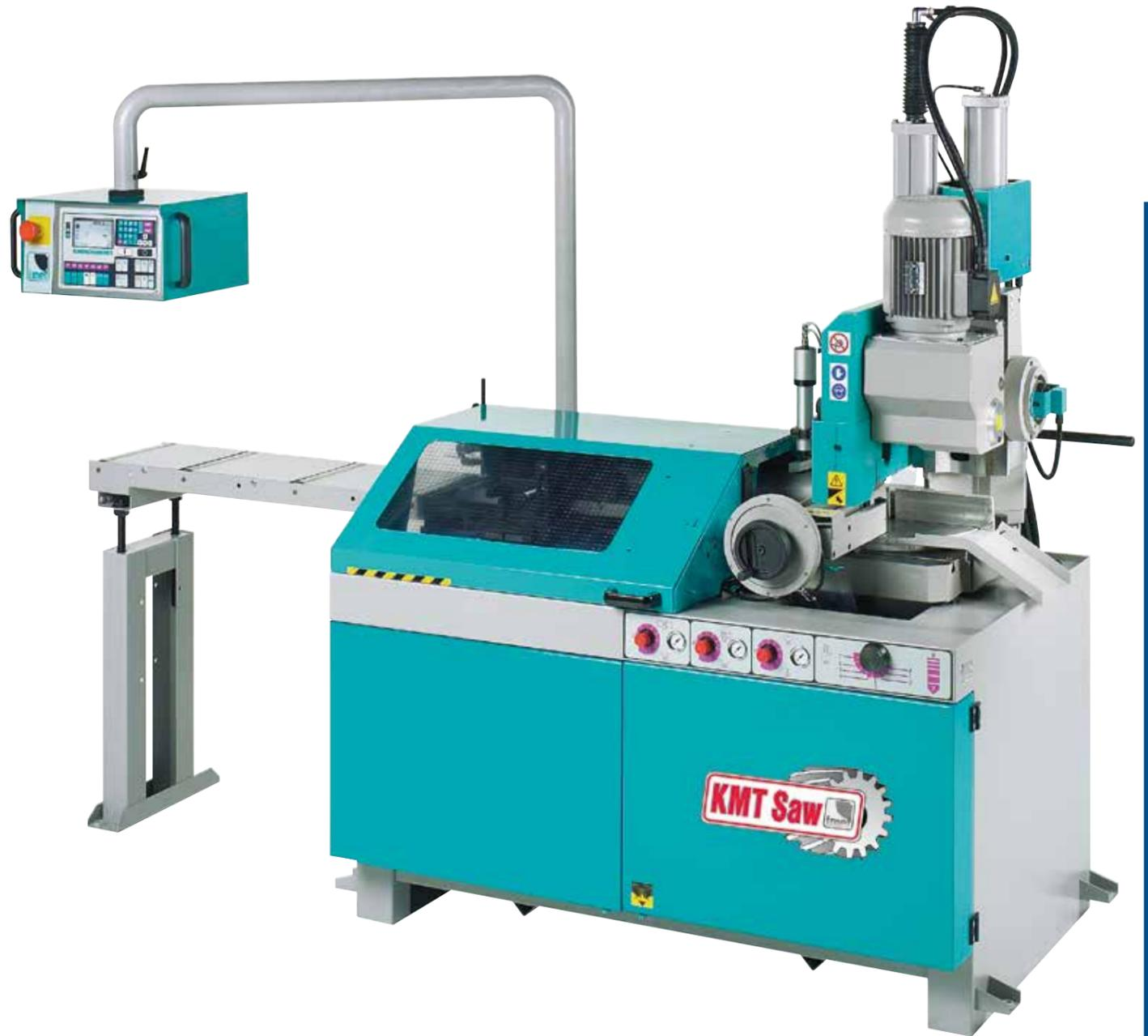
We offer an extended feeder option which is faster and brings the index length to 47"
