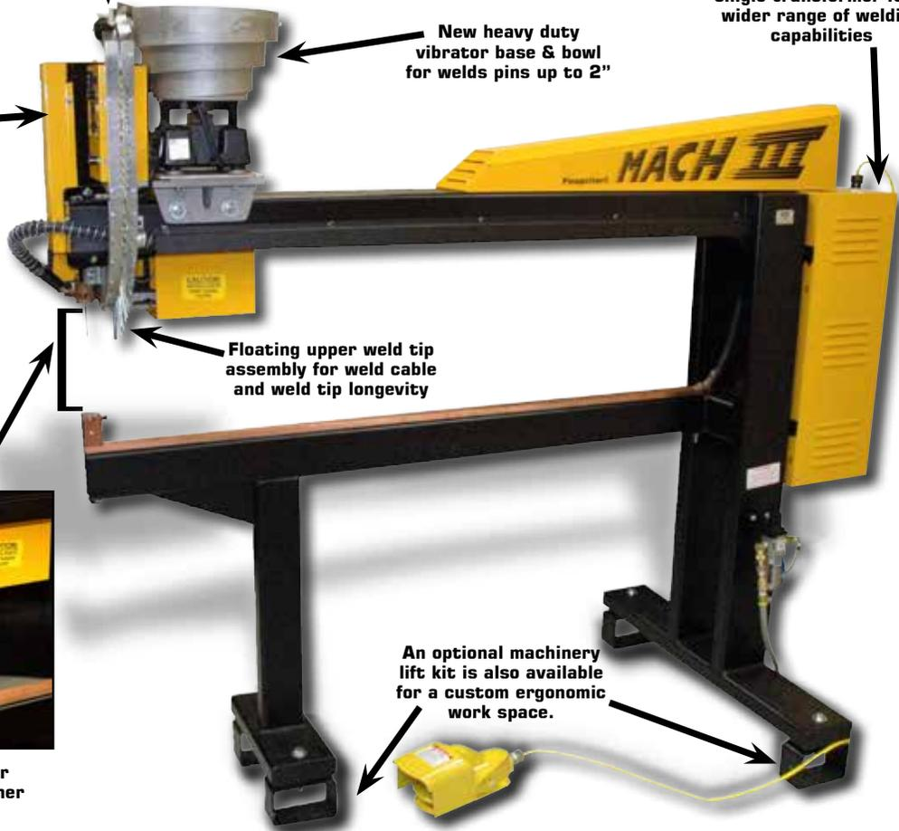
Floating upper weld tip assembly for weld cable and weld tip longevity
