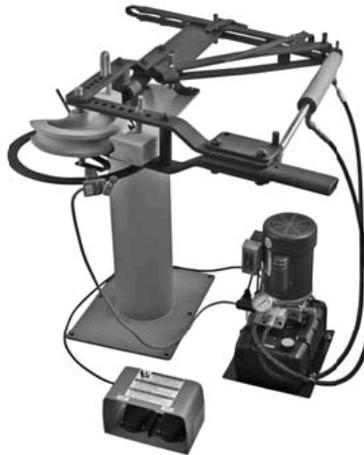
This is the best value-this hydraulic package includes everything you need to use hydraulic power for most applications. Includes: H60 Hydraulic Power Unit, double-action hydraulic cylinder, hoses, foot switch, and conversion kit to convert the Model No. 2 Bender for use with hydraulic power. Bend offsets, angles, return bends, or 360° circles with most tooling, as appropriate.
